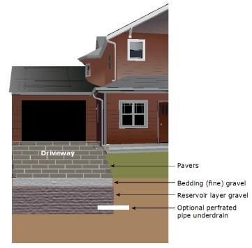
Existing soils that allow infiltration at 1 inch per hour minimum if soils do not have a lot of clay, preferably 2 inches per hour.
